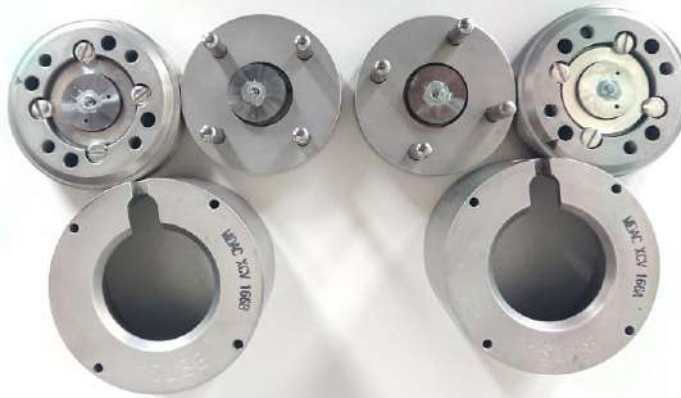
Figure. 21 Photographs of MDAC for High pressure XRD and Raman measurements up to 20 GPa.
