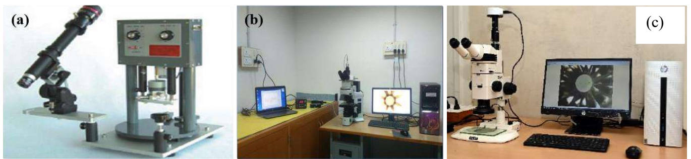
Figure 9: Photograph of (a) micro drilling machine; (b) Ruby fluorescence P calibration setup; (c) Stereo zoom microscope for sample assembly.
