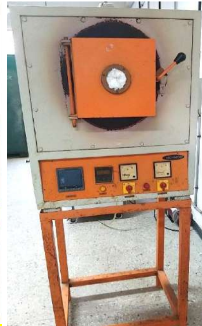
Muffle Furnace (Technico, Chennai) up to 1200°C
