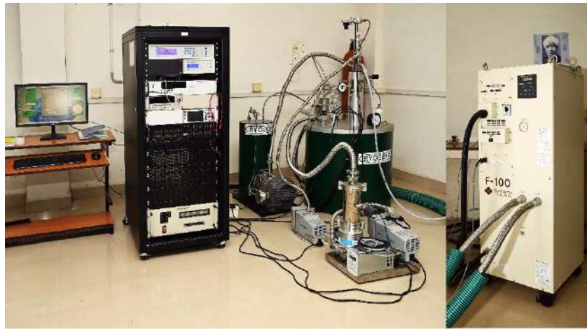
Figure 19. 9T cryogen free superconducting magnet with an Integrated Variable Temperature Insert (IVTI) (Cryogenics, UK) with measuring instruments and power supply for a magnet.
